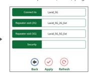
Select the SSID of the target network and insert Repeater SSID and the key of your network. the default Repeater SSID is set to be xxxx\_2G\_Ext / xxxx\_5G\_Ext (xxxx indicates The Main Router's wireless network name). Then click Apply to complete setup.
