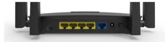
**WPS Button:** If your Wireless Adapter supports WPS function, you can press the WPS button and then press the WPS button to establish a secure connection between the Wireless terminal devices and the AC Router.
